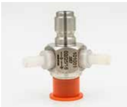
Part # IN-101031 Description General .057 Injector 2 Barb - Kynar Quick Con. With 0.057" Orifice - 1.0 GPM
