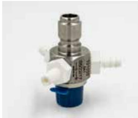
Part # IN-101035 Description General .041 Injector 3 Barb - Kynar Quick Con. With 0.041" Orifice - 0.5gpm
