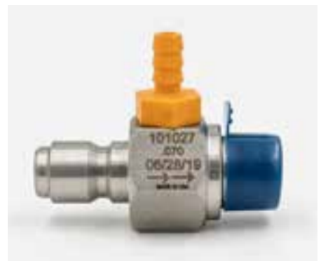
Part # IN-101027 Description General .070 Injector 1 Barb - Kynar Quick Con. With 0.070" Orifice - 1.4 GPM
